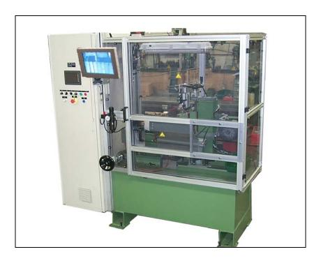
Armature load-unload: manual between centres
